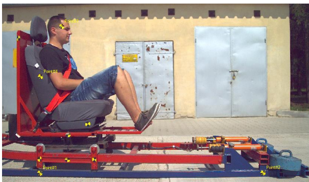
Fig. 3. The diagram of the testbed for collision tests [9]
