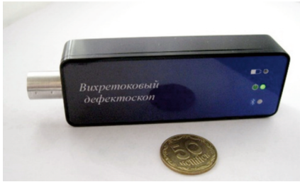
Figure 5. The transducing unit of the ECNDT system.
