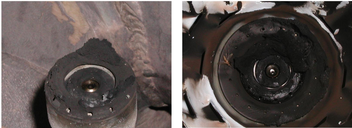
Fig. 1. Carbon deposits on jet engine injectors (photographs taken during engine overhaul) [1]
