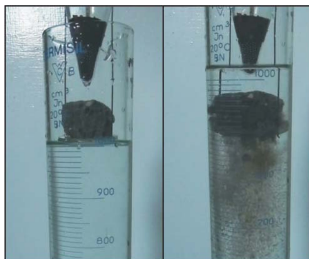
Fig. 12. Soaking of a grey-brown brick: left photograph – sample prior to inserting in water, right photograph – desintegration of a sample after inserting in water.
