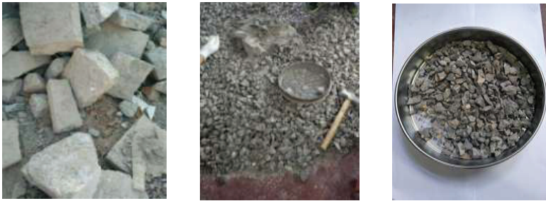
(a) Waste concrete (b) Breaking waste concrete (c) Screening coarse aggregate
