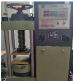
(c) YA-2000 digital display pressure tester
