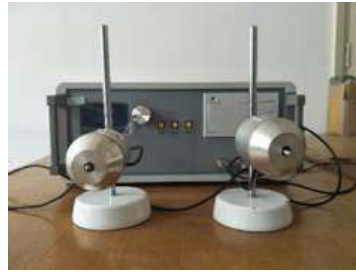
(b) DT-20W dynamic modulus of elasticity of tester
