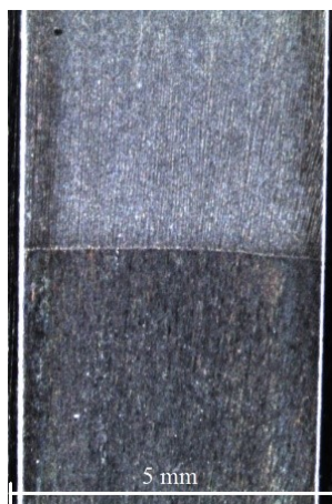
Fig. 2. Solidification front in Fe-4.25%C sample of 5 mm diameter, solidified directionally at 125 μm/s and G=33.5 K/mm, x 2
