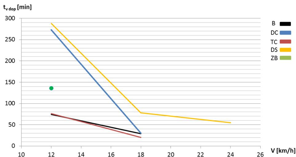
**Fig. 12.** Influence of the driving speed on the value of the allowable duration of the vibration impact for the substrates under testing
