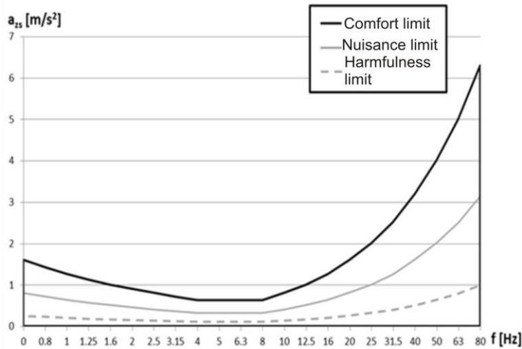
**Fig. 1.** Limits of comfort, nuisance I harmfulness in the vertical direction, where:  $a_{zs}$  – the effective acceleration towards Z.
