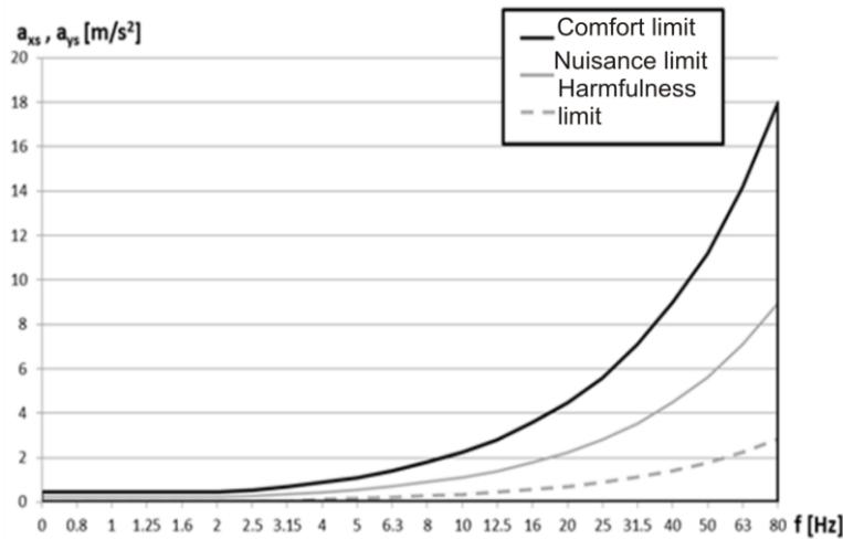
**Fig. 2.** Limits of comfort, nuisance I harmfulness in the horizontal direction, where:  $a_{xs}$  – the effective acceleration towards X,  $a_{ys}$  – the effective acceleration towards Y.
