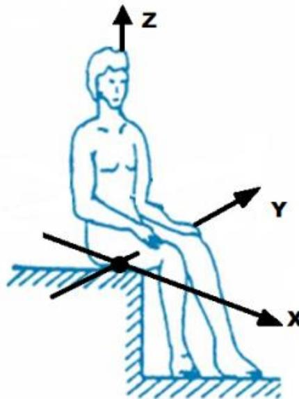
Fig. 7. Diagram of the accepted reference system for the measured acceleration components
