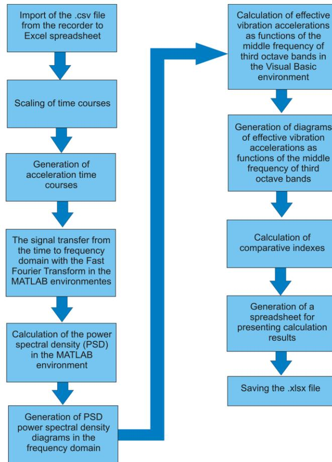
**Fig. 3.** The block diagram of the algorithm operation for determining the characteristics and comparative indicators of vehicle driving comfort
