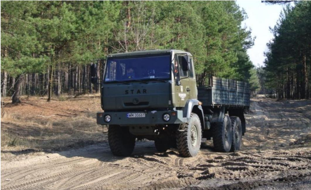
**Fig. 4.** View of the Star 1466 vehicle during the road test in the military training ground roads (tank road No. 2)
