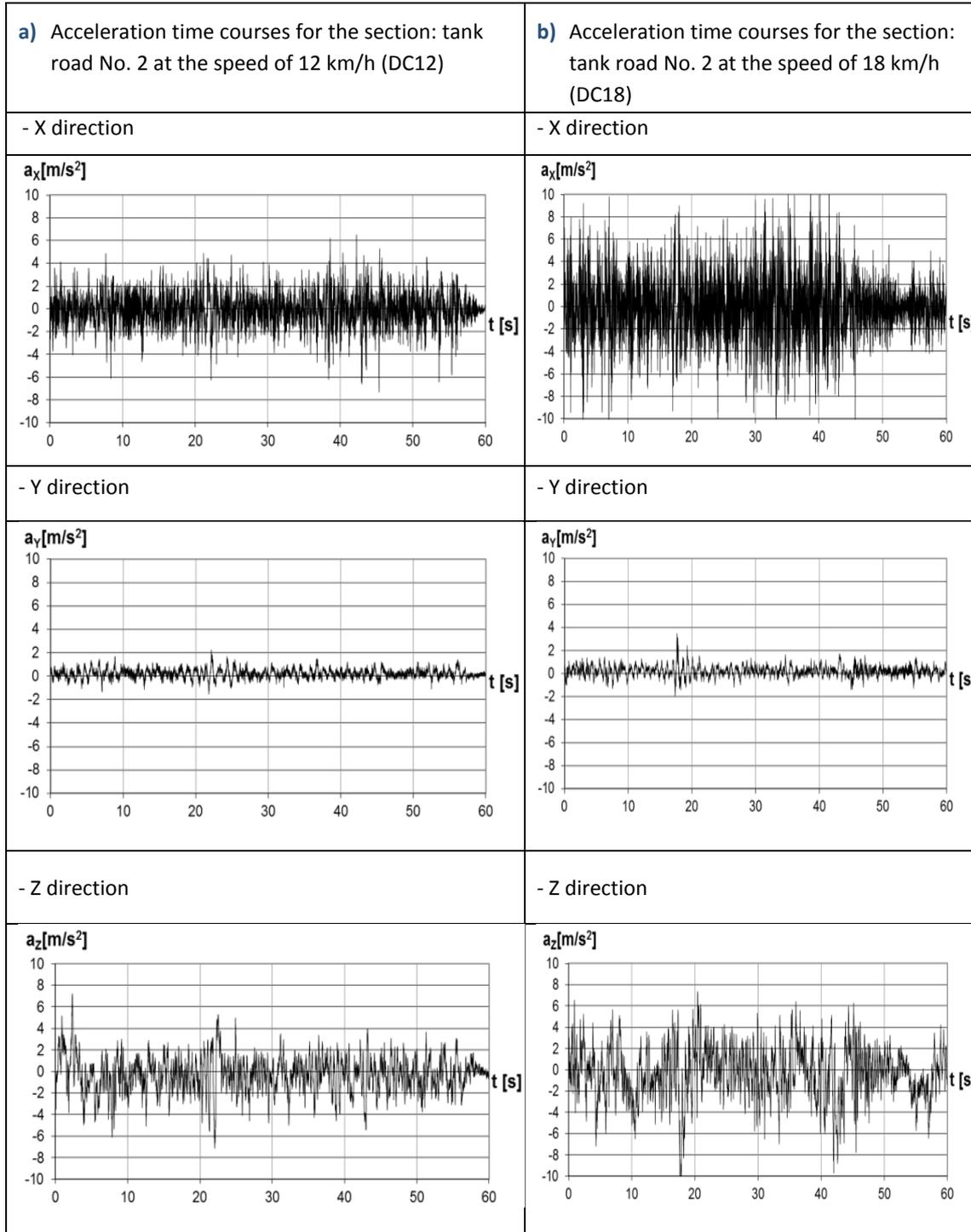
**Fig. 10.** View of the exemplary results of the acceleration time courses for two different speeds on the same substrate
