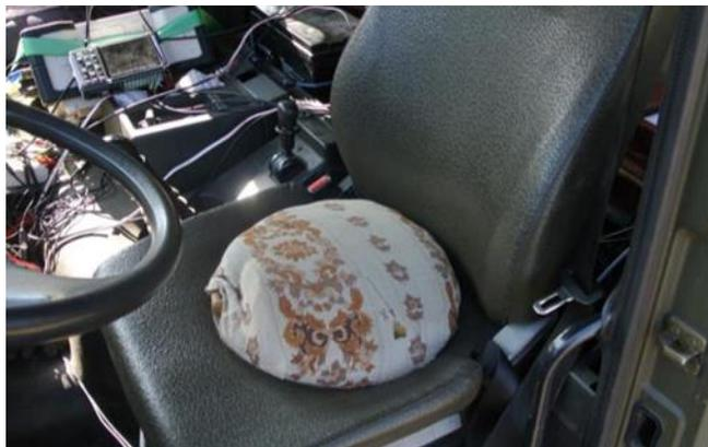
**Fig. 9.** View of the measuring disc (cushion) with a mounted triaxial acceleration sensor installed on the driver's seat
