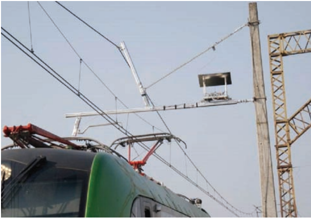
Fig. 28. Traction vehicle passage under tested OCL cantilever system with raised one (left) and two (right) pantographs [photo P. Kwaśniewski]
