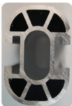
Fig. 4. Shape of an aluminum alloy EN-AW 6082 profile used as a main profile, cantilever support, registration arm [5, pp. 429-436]
