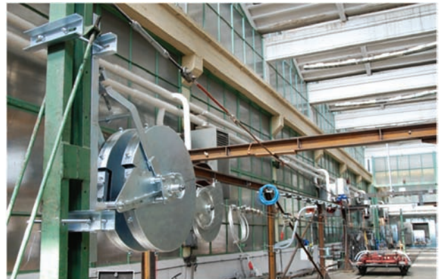
Fig. 22. No-load tensioning device during laboratory tests [photo P. Kwaśniewski]
