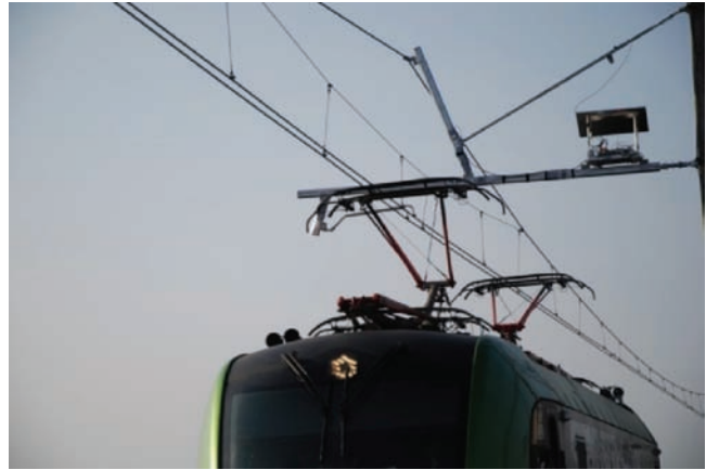
Fig. 28. Traction vehicle passage under tested OCL cantilever system with raised one (left) and two (right) pantographs [photo P. Kwaśniewski]
