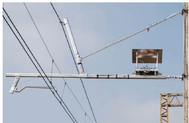
Fig. 27. Tested OCL cantilever system with visible mounted strain gauges and measurement equipment [photo P. Kwaśniewski]
