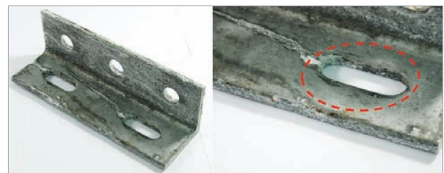
Fig. 13. An anchor holder after 24 hours of salt fog exposure [8, pp. 421-428]
