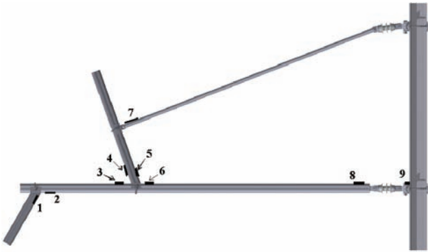
Fig. 14. Overhead contact line new generation accessories mounted on the pole with tension measurement areas marked [11]
