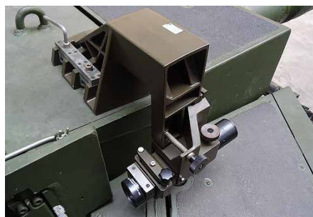
Fig. 3. Measuring instrument for bore-sighting gunsights
