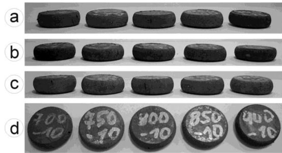
Fig. 5. Appearance of Cu-3Ti alloy specimens after compression at temperature in the range 700\div 900^\circ\text{C} up to a strain of 1.2 (70%) with strain rate of 0.1 (a), 1.0 (b) and 10.0\text{ s}^{-1} (c)
