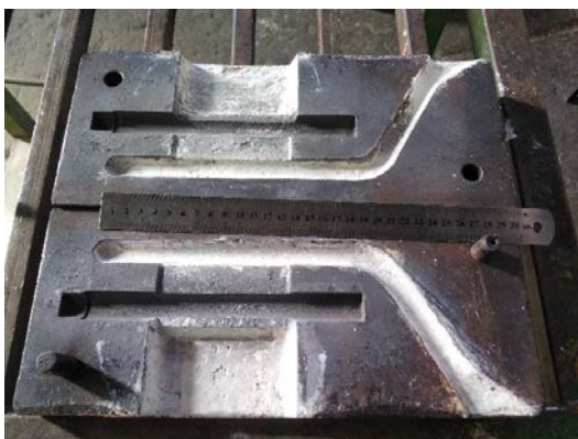
Fig. 2. The geometry of the casting mold
