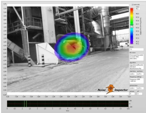
Fig. 6. Source Z2 (industrial fan) – flow Q = 14\,000\text{ m}^3/\text{h} , diameter 1 m, frequency range 230–250 Hz.
