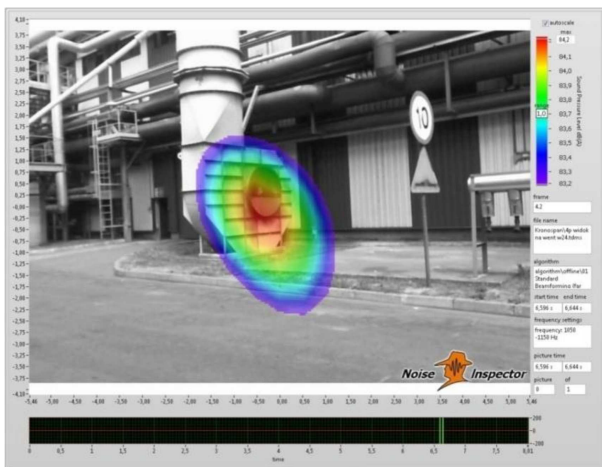
Fig. 8. Source Z3 (industrial fan) – flow Q = 120\,000\text{ m}^3/\text{h} , diameter 1.3 m, frequency range 110–120 Hz.
