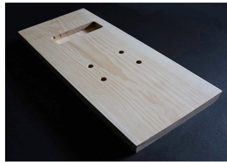
Fig. 1. Raw wood element for solid body of electric guitar with routed pickup- and bridge holes.
