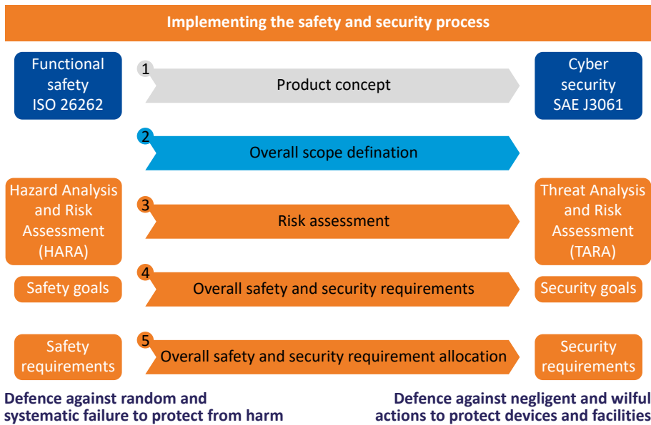
Fig. 2. Implementation of a safety and security process
