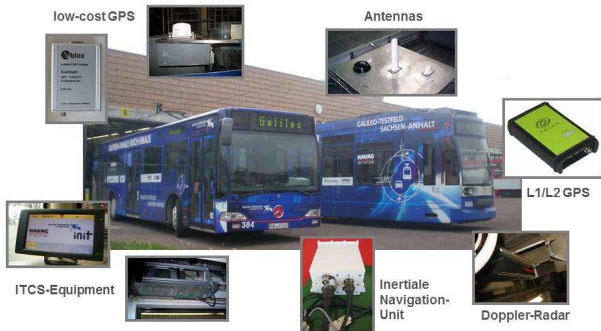
Fig.1. Scientific development platform consisting of PT vehicles and high performance sensor equipment
