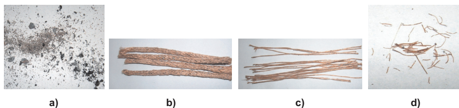
Fig. 4. The solid residue of gasification experiment: a) non-metallic residue (with small pieces of copper), b) copper braids, c) cooper cords, d) pieces of cooper manually separated. Copper cords were removed from copper braids after experiment, for better presentation
