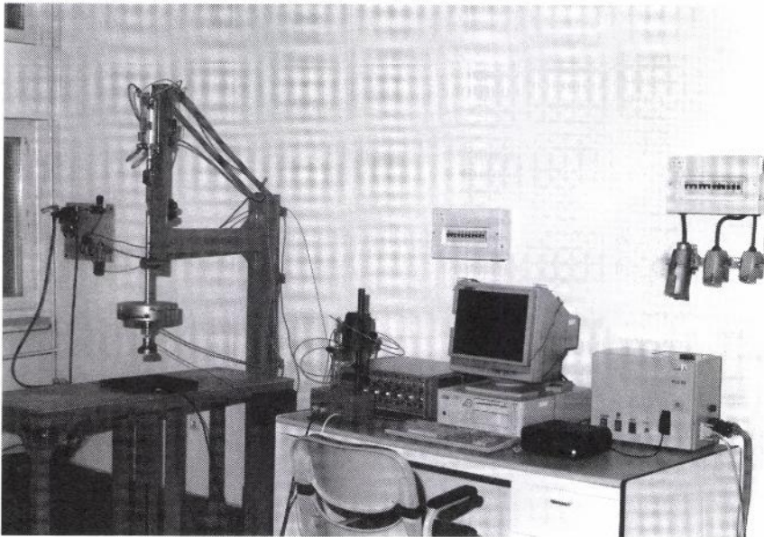
Figure 1c. Test stand A for measuring the actuating force, response time, and static pressure resistance.
