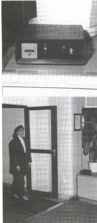
Figure 13. A functional test of a pressure sensitive mat.
