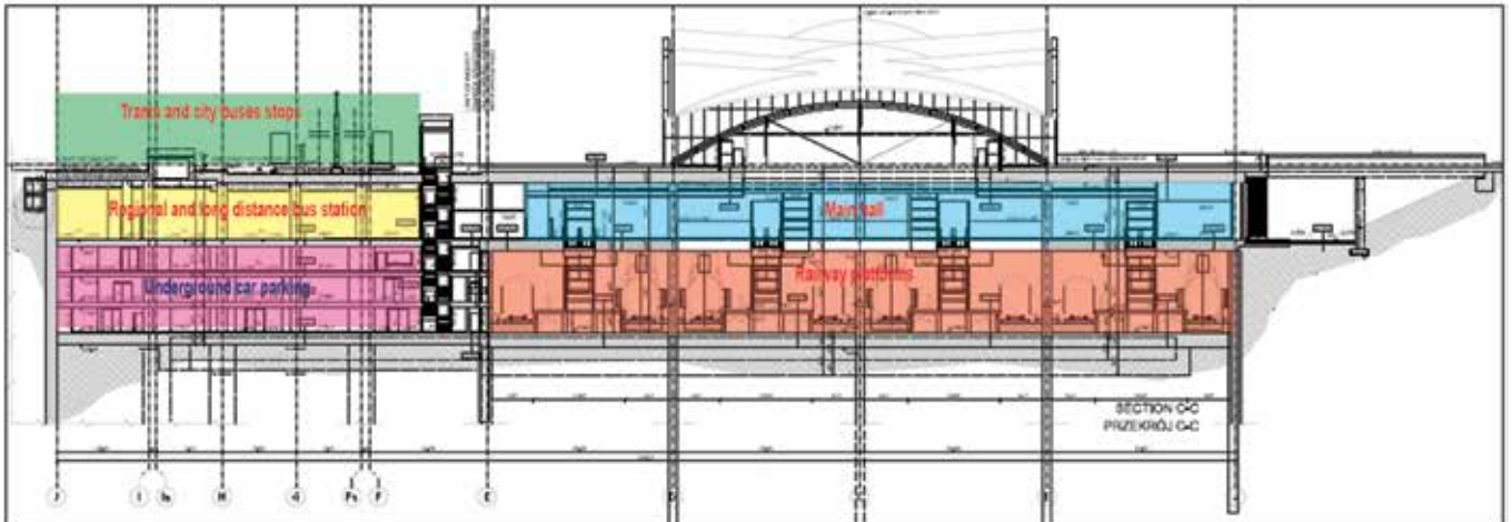
Cross-section of the planned Łódź Fabryczna station – view from the west entrance
