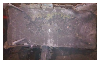
Fig. 7. Casting containing 0,95 kg of electrocorundum grains
