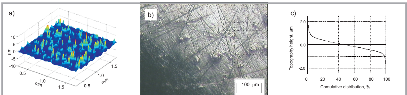
Figure 9. Stereometric structure of the burnished surface of the spindle-neck coating, made of aluminum alloy AlCu4Mg1, after about 21600 hours of working contact with yarn (on the border of the helical groove): a) surface topography: S_a = 0.40 \mu\text{m} , S_q = 0.53 \mu\text{m} , S_p = 6.77 \mu\text{m} , S_t = 11.73 \mu\text{m} , S_k = 2.06 \mu\text{m} , S_{pk} = 0.16 \mu\text{m} , S_{vk} = 0.54 \mu\text{m} ; b) microphotograph of the surface, c) curves of the surface material part.
