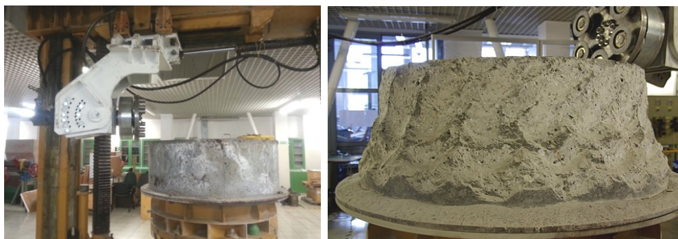
Fig. 8 The view of modernized test stand and view of mining test for one of the disk tool sets Source: (Kotwica et al. 2017)
