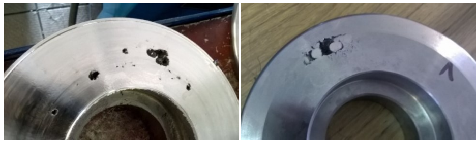
Fig. 12 A view of defective copies of disk tools made of cast steel
