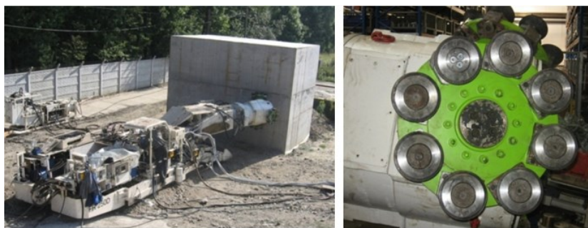
Fig. 10 A view of FR250 road header with mining head with disk tools
