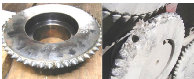
Fig. 11 View of disk tool reinforced with sintered carbide inserts and traces of carbide inserts breakage
