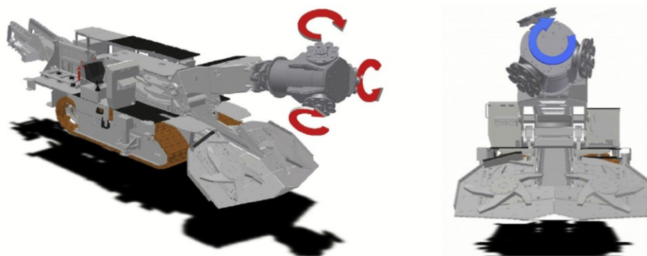
Fig. 9 Scheme and kinematic capabilities of the new head mounted on the roadheader KR 150
