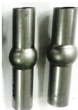
Fig. 7. Examples of the hydroformed specimens obtained experimentally
