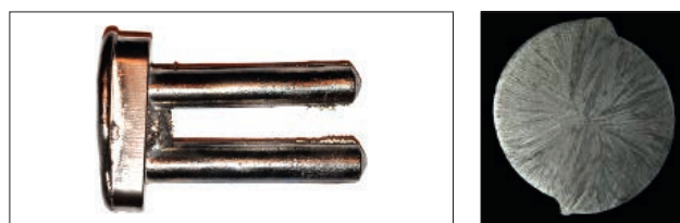
Fig. 1. Test material from cobalt Co-20Ni-10Al-5Mo-2Nb superalloy: a) superalloy cast, b) cross-section through the cast bar
