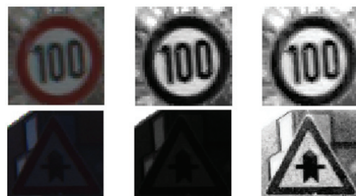
Fig. 2. Two examples of preprocessing stages (in each row): original image, after RGB to gray conversion and intensity adjustment and after histogram equalization, respectively
