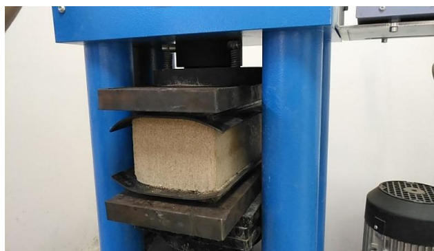
Fig. 3. Compressive strength test preparation
