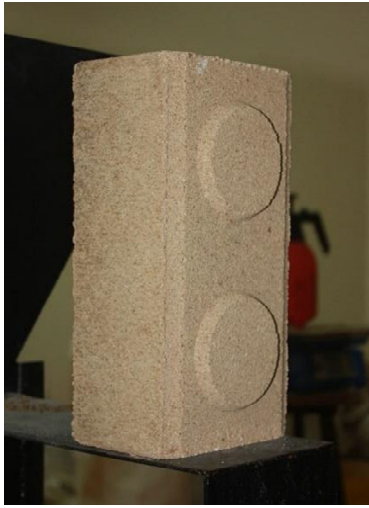
Fig. 1. 300×150×108 mm block dimension
