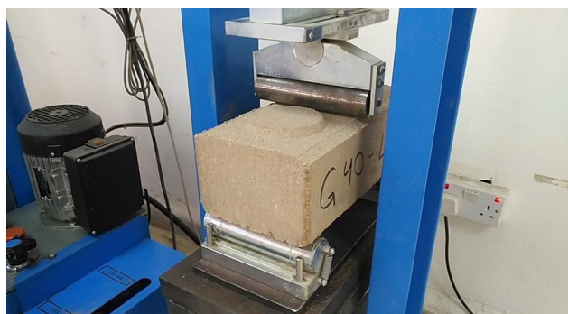
Fig. 4. Flexural strength test preparation
