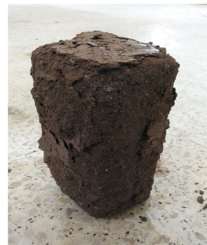
Fig. 15. BL mix specimen after getting out of water
