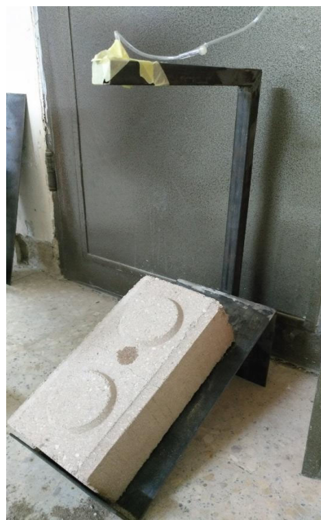
Fig. 5. Geelong drip test
