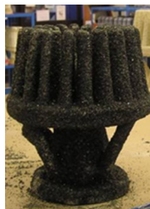
Fig. 1. The pattern assembly with 20 airfoil blade castings
