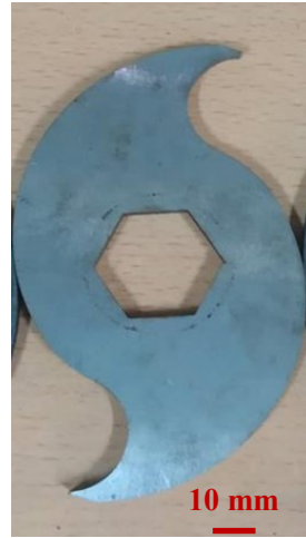
(b) photograph of a fabricated shredding blade
