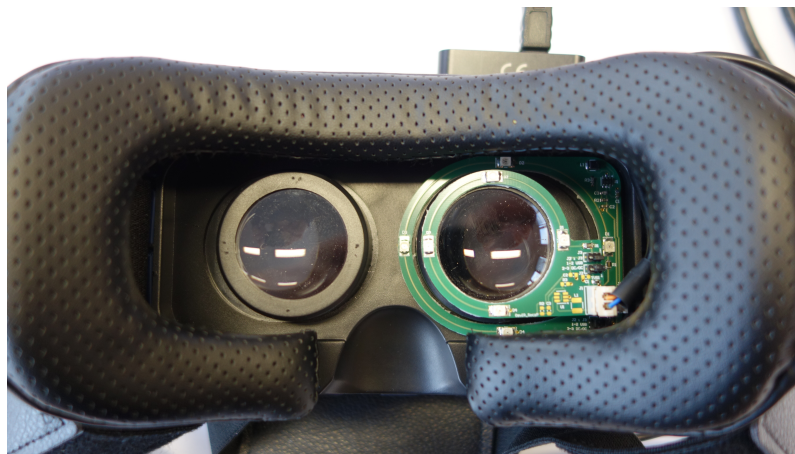
Fig. 3. Developed model of the device to record eye movements using a camera working in the near infrared - rear view.
