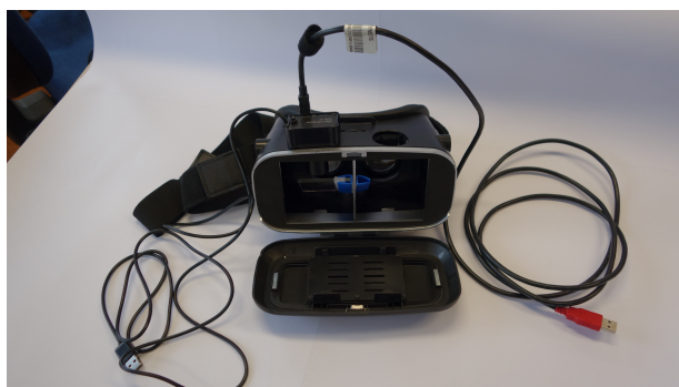
Fig. 2. Developed model of the device to record eye movements using a camera working in the near infrared - front view.
