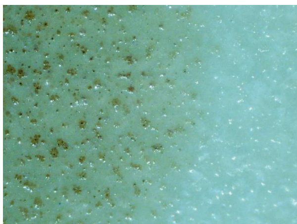
Image 7. Area of sample J1 where water droplets were applied and which was exposed to UV radiation for 20 minutes and then to a solution of H_2S (left side) and UV radiation for 30 minutes (right side)
