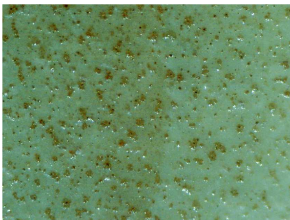
Image 6. Grey area on J1 sample in place of application of water droplets after UV exposure for 30 minutes followed by exposure to an H_2S solution.
