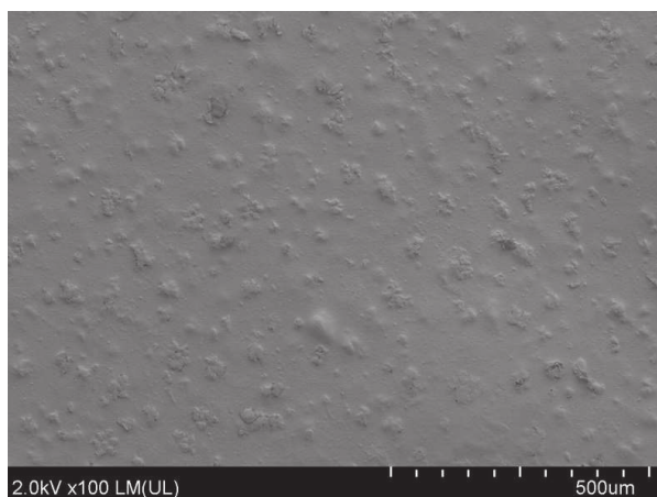
Image 2. SEM image – fragment of J1 sample surface exposed to UV radiation without the presence of H 2 O
