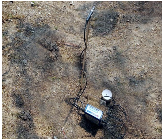
Fig. 11. Seismograph measuring the ground vibration
