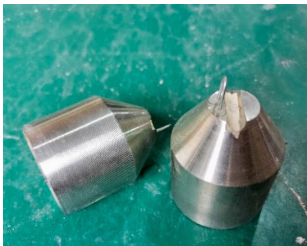
Figure 3. The physical picture of the shaped charge device
