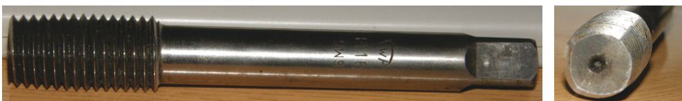
Fig.4. Burnishing screw-tap M16 made joint similar to rolling screw
