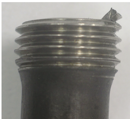
Fig. 7. View from the side for the cracked double – nutted bolt
