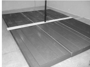
Fig. 2. Sample No. 3 of sound-absorbing panels of aluminium sheet perforated and profiled.
