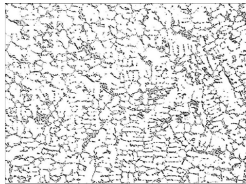
Fig. 1. Microstructure of the remelted AlSi9Mg alloy, magn. 100 \times
