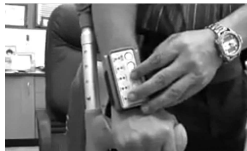
Fig. 11. Control panel of the ReWalk device [17]
