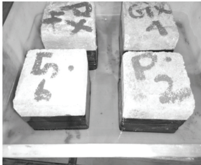
Fig 7. Sorptivity test specimen
