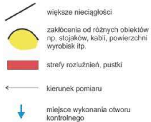
Rys. 5. Objasnienia symboli na radarogramach Fig. 5. Explanations of symbols for radarograms
