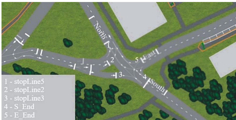
Fig. 8. The intersection configuration in the model without traffic light control (Source: own work)
