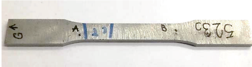
Fig. 2. Specimen 523 4B with marked (A, B, C) discontinuities of the internal structure subjected to ET tests.
