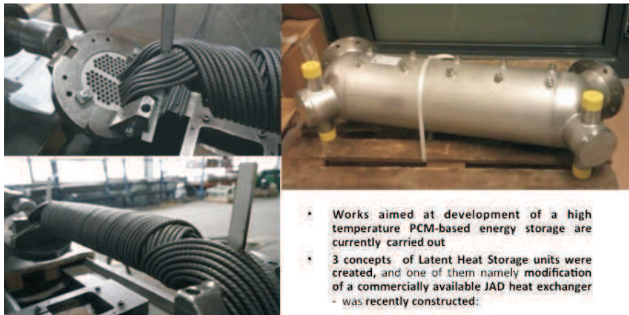
Figure 13: PCM-based energy storage prototype in the lab in the IMP PAN (testing rig is currently under construction).
