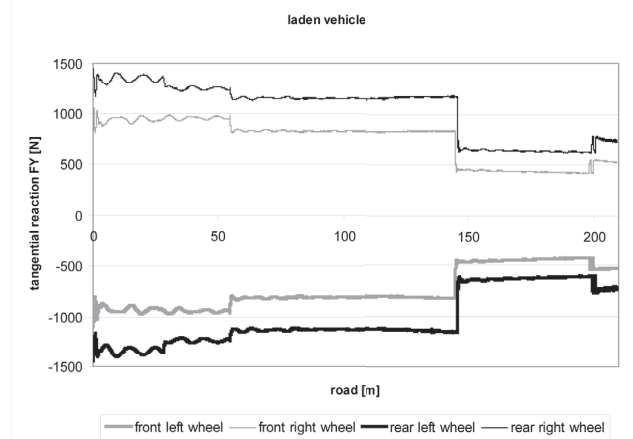
Fig. 3. Courses of the tangential reaction forces (FY components) on the flat and dry road [own study]
