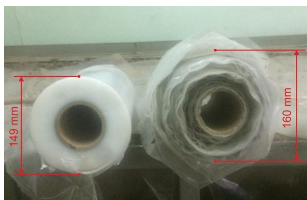
Fig. 12. Compacted bundle of used plastic mulch (right) compared to the standard mulch bundle (left) (phot. K. Khazimov)
