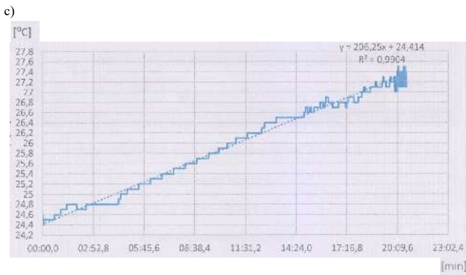
Fig. 7. Results of the measurements of the temperature of lapping disc in idle mode: a) in the initial moment, b) after 20 min ( n = 40 \text{ min}^{-1} ), c) graph showing the increase of the temperature of the lapping disc in time (on average, 0.14^\circ\text{C}/\text{min} )
