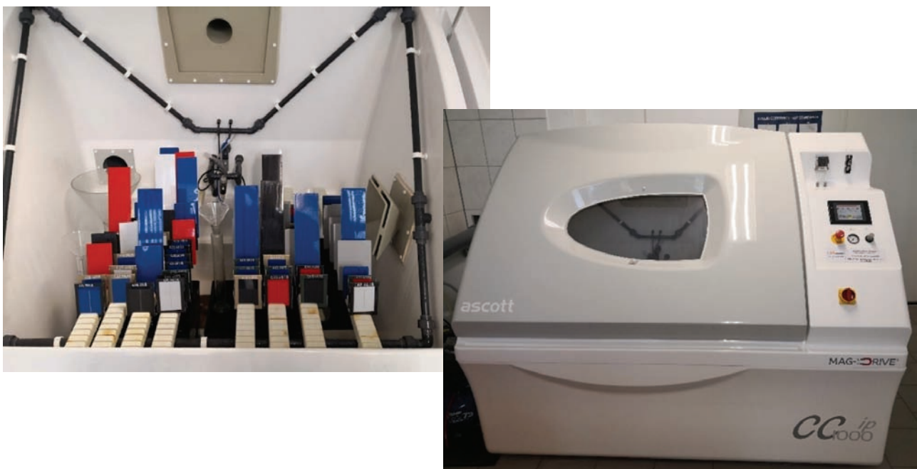
Fig. 3. Test stand for ageing samples according to PN-EN ISO 9227 [12] (Ascott CC1000IP salt spray chamber) [Pic. M. Garbacz]
