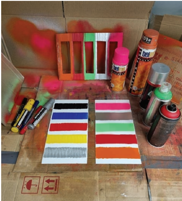
Fig. 4. Test stand for determining graffiti resistance [Pic. M. Garbacz]
