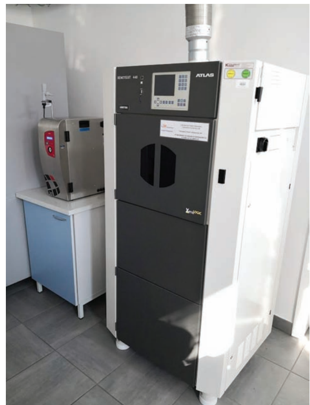
Fig. 1. Test stand for ageing samples according to ISO 16474-2 [7] (xenon weathering instrument, Atlas GmbH Xenotest 440) [Pic. M. Garbacz]
