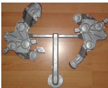
Fig. 10 Non-machined casting with a gating system
