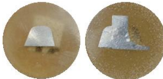
Fig. 13 Specimens intended for grinding and polishing for optic microscopy
