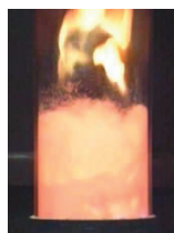
Fig. 5. The fluidised bed combustion of propane with some polycarbonate sample (bed temperature 900°C)
