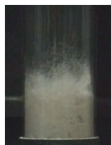
Fig. 3. The fluidised bed reactor just after the ignition of propane-air mixture (bed temperature 400°C)
