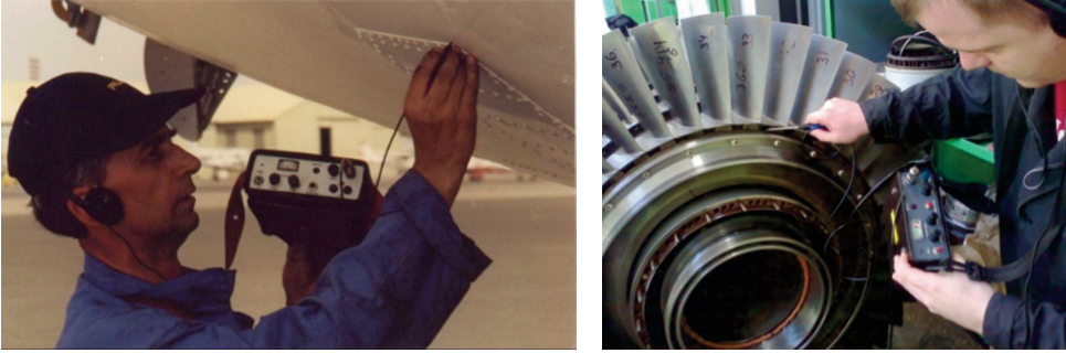
Fig. 10. Inspection of AN-12 aircraft fuselage (a) and engine components (b) by the VD3.03 type EC flaw detector.
