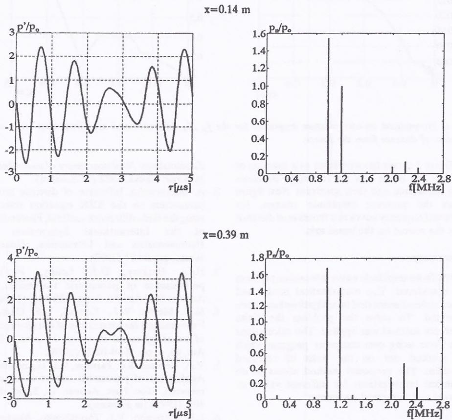
Fig. 5. The waveform as a function of time on the beam axis for fixed distances from the source and the spectrum corresponding to it.
