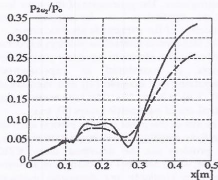
Fig. 3. Normalized on-axis pressure amplitude for  $f_2$  and  $2f_2$  frequency wave as a function of distance from the source for different values of step size  $\Delta x$ .
