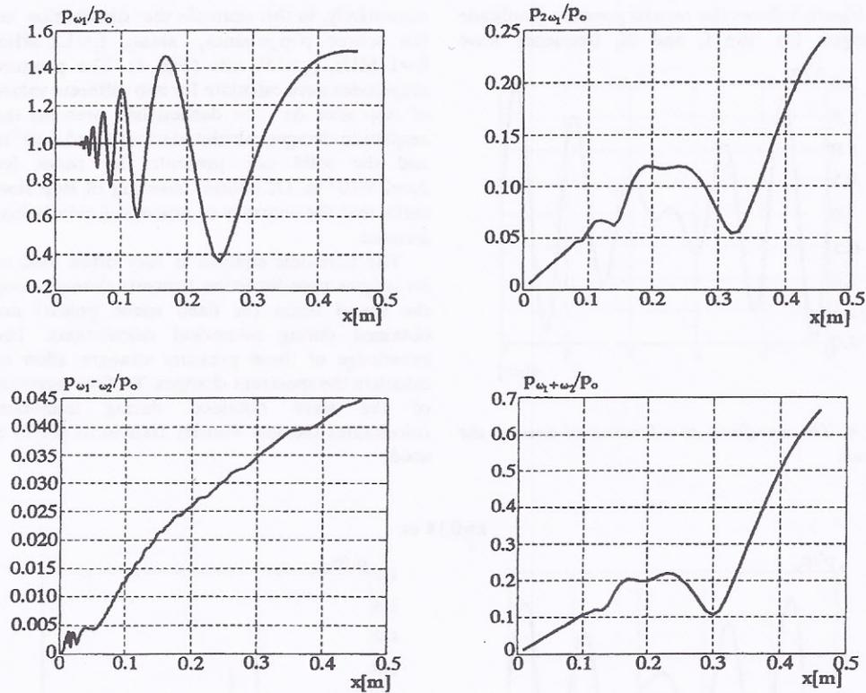
Fig. 6. Normalized on-axis pressure amplitude for the  $f_b$ ,  $2f_b$ , difference and sum frequency wave as a function of distance from the source.
