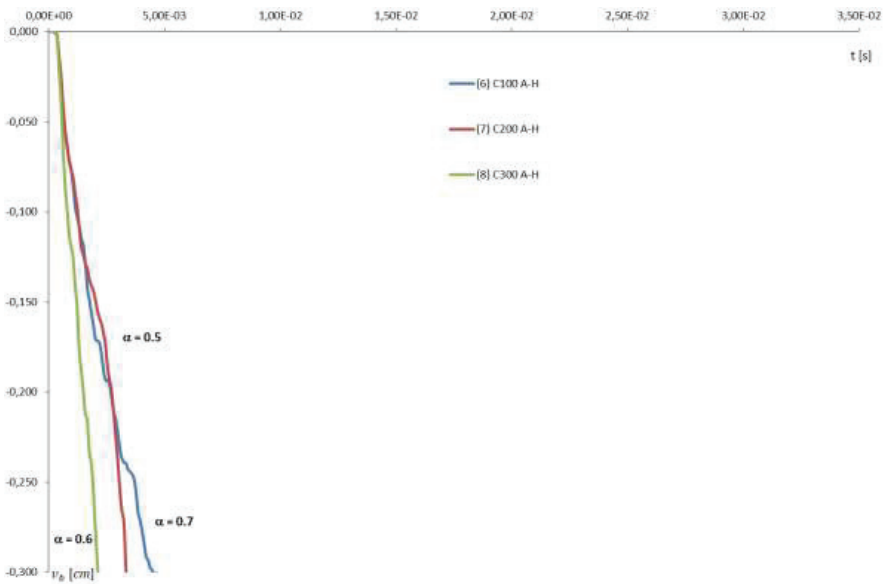
Fig. 8. Variation in time of displacement of midpoint x_b at the bottom edge for the load levels corresponding to the destruction phase
