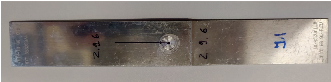
Fig. 3. Specimen I1 representing the initial state after the RFSSW process with following parameters: spindle speed – 2200 rpm, tool plunge depth – 1.5 mm, duration of welding – 2.5 s.
