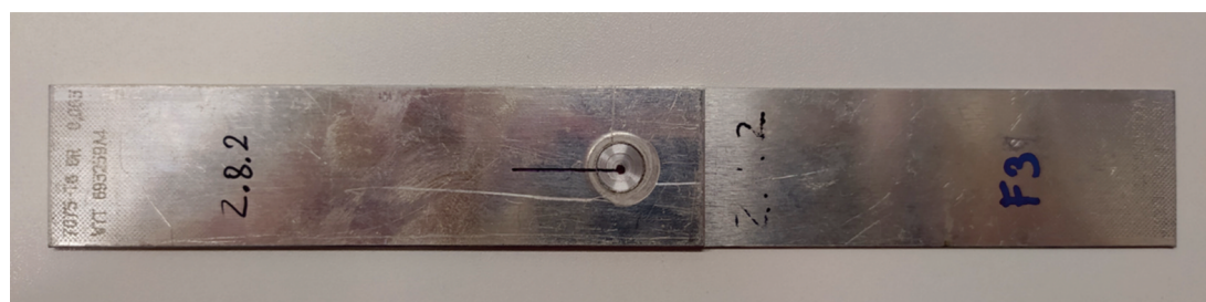
Fig. 7. Specimen F3 after the fatigue tests: maximum force – 1 kN, 17 \cdot 10^3 fatigue cycles.
