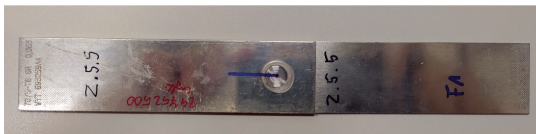
Fig. 5. Specimen F1 after the fatigue tests: maximum force – 0.9 kN, 25 \cdot 10^6 fatigue cycles.
